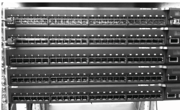
Figure 3.2: Juniper Networks EX4200 mounted in the lab
